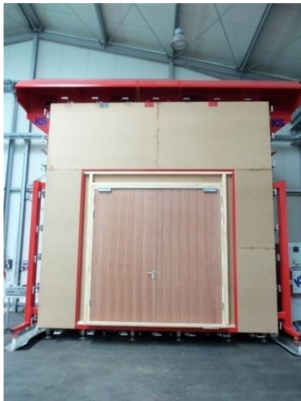
Chamber for smoke leakage tests 5 x 5 m – front view; example for reduction in size to 3,4 x 3,4 m
