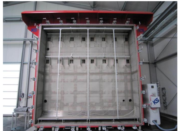
Chamber for smoke leakage tests 5 x 5 m – interior view
