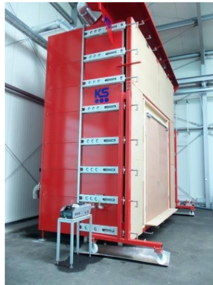
Chamber for smoke leakage tests 5 x 5 m – side view
