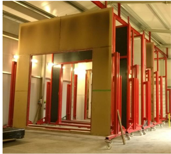
Test hall repeated opening and closing
