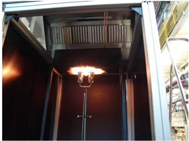
Flame resistance testing in accordance with LPS 1263
