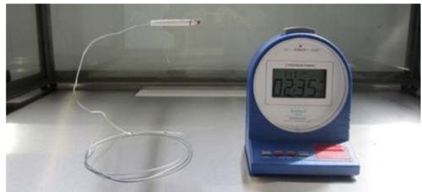
Test preparation: smouldering cigarette test
