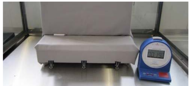
Test setup upholstered furniture: smouldering cigarette test
