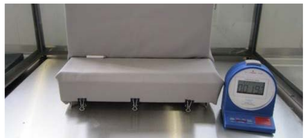
Test setup upholstered furniture: smouldering cigarette test
