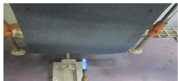
Setup for flame application to the edge of a curtain
