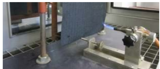
Flame application to the surface of a curtain
