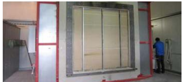
Vertical furnace 4 x 4 m – Downsizing to 2.44 x 2.5 m (W x H)
