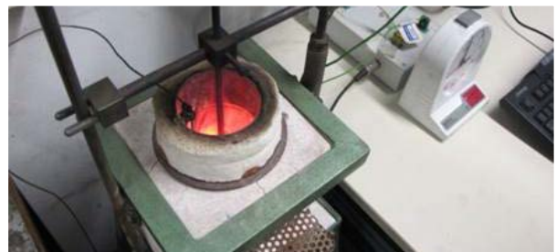
Progress of fire test in the Non-combustibility test furnace
