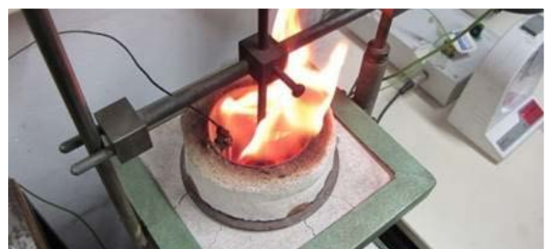
Reaction of sample material in the Non-combustibility test furnace
