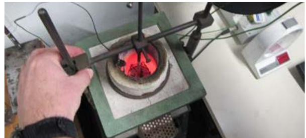
Start of fire test in the Non-combustibility test furnace
